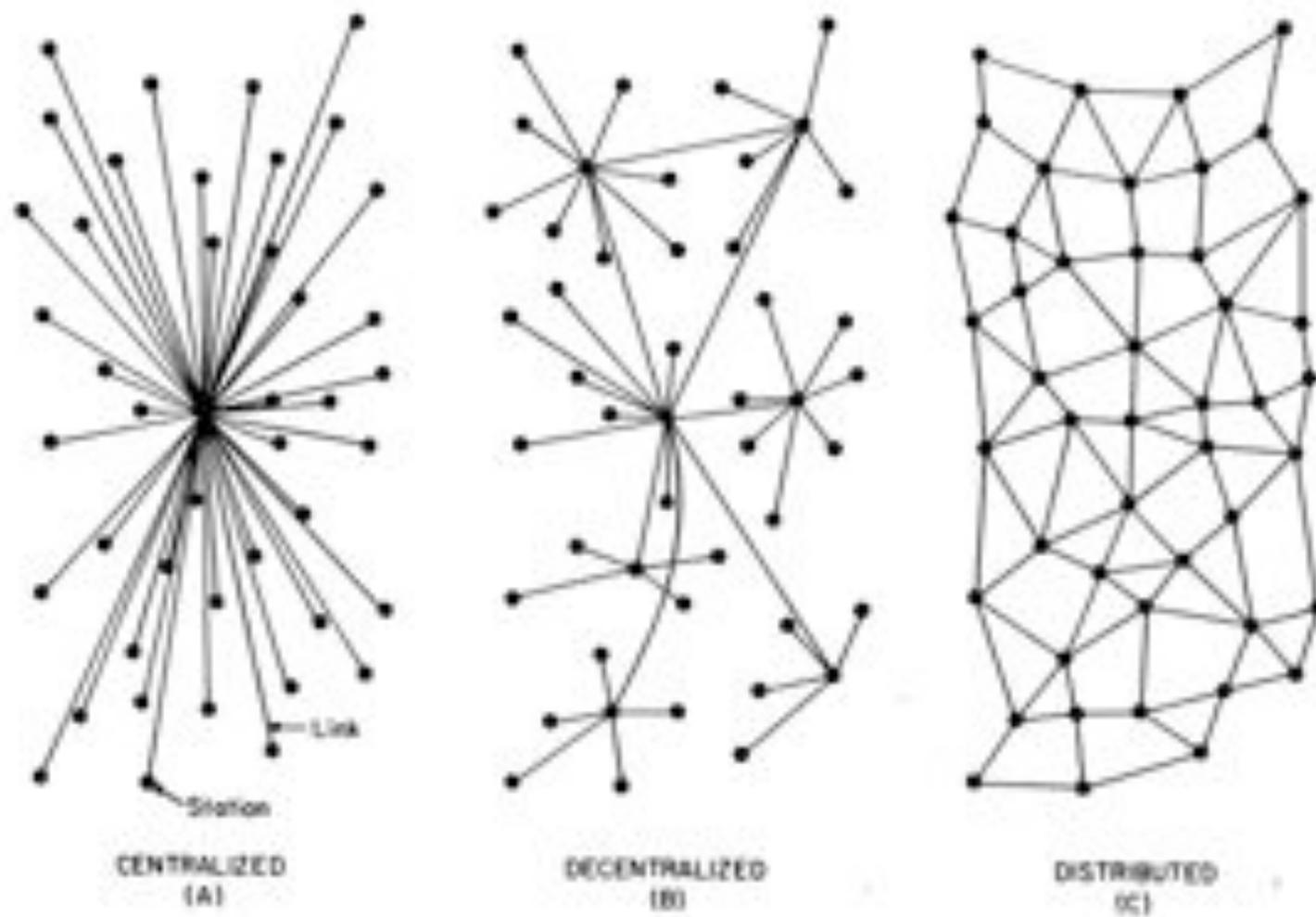
FIG. 1 - Centralized, Decentralized and Distributed Networks
